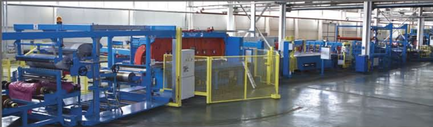
The carvass and steel belts cutting line made by Fischer, Germany.
